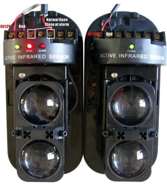
To connect the Active Infrared Sensor to IP CAMERAR camera ALARM IN, will trigger alarm when light beams interrupted.
