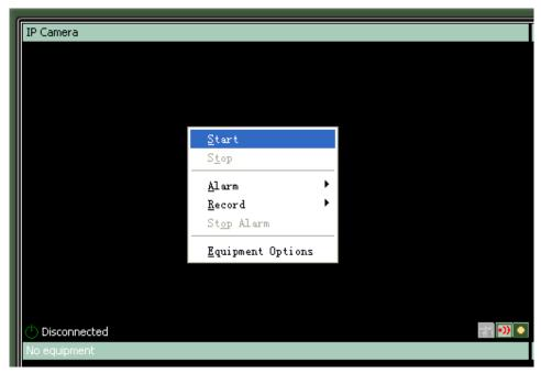
Right click within the window, an operation menu will come up. Or click one of the three buttons at the lower right corner to setup snapshot, alarm, or video record.
