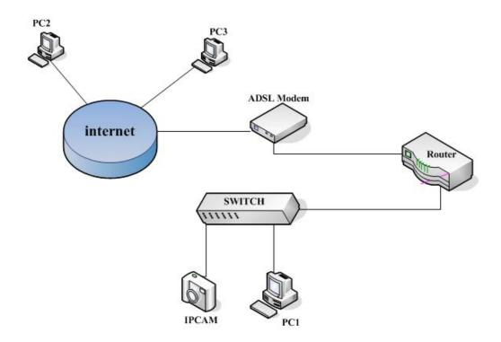
Connection of IPCamera and Network: Before using SuperIPCam, connect IPCamera to net. You can connect the IP camera into LAN, or connect into LAN then to the internet by ADSL Modem. Please refer to the chart above.
