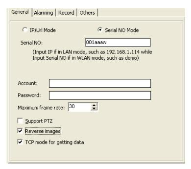
Note: "TCP mode for getting data". If not Checked, when more than 1 user is visiting the IPCamera simultaneously, User end might request data from other users so as to reduce the work load of the IPCamera. But this might make the data stream not stable. Users make their choice.
