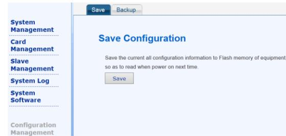
**Function Explanation:** Save all master configurations and won't be deleted if power failure.
