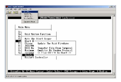
4. Select "ZMODEM modem" under Protocol to set ZMODEM as the file transfer protocol of your terminal emulation software.
