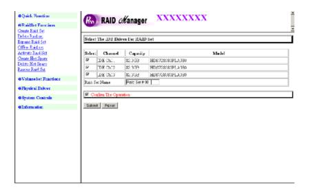
To create a Raid Set, click on the Create Raid Set link. A "Select The IDE Drives For RAID Set" screen is displayed showing the IDE drives in the RAID subsystem. Check the "Select" option to include a physical drive to the current Raid Set. Enter the preferred Raid Set Name (1 to 16 alphanumeric characters) to define a unique identifier for the Raid Set. The default Raid Set name will always appear as Raid Set # 00 for first Raid Set.
