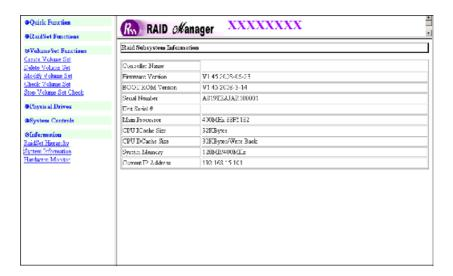
The controller name, firmware version, serial number, main processor, CPU data/instruction cache size and system memory size/speed appear in this screen.
