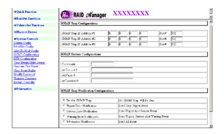
SNMP Trap Configurations: Type the SNMP Trap IP Address. The SNMP Port is set to 162 by default.
