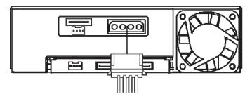
Step 3 Connect one end of the SATA cable to the SATA port on the product body and the other end to the SATA port on the motherboard
