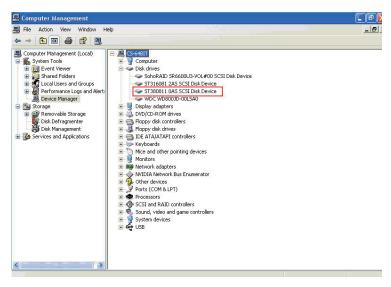
Step 2 Select the newly added HD drive, and start initializing the HD. After the initialization is done, you can "format" the HD as a desired one according to your preference or need. After the formation, you can start using the HD device
