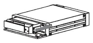
Step 6 Insert the encryption key into the encryption key slot in front of the product body properly
