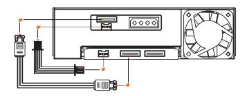
Step 2 Install the product body on the computer, fasten it with the screws that come with the accessory kit, and then connect the power cord
