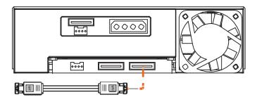
Step 4 Remove the tray and fasten the HD drive with the screws that come with the accessory kit
